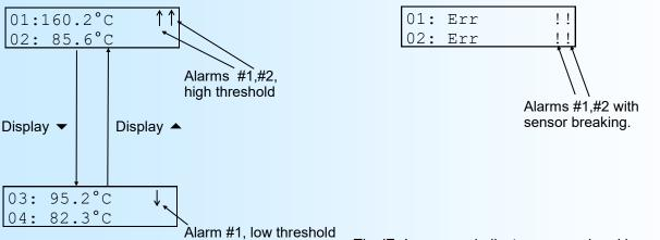
The 'Err' message indicate a sensor breaking error.
