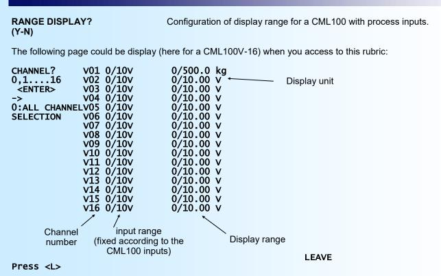
To change the input parameters for the channel, enter the channel number and press <Enter>. The number '0' is for a configuration for all channel. Press <L> to quit the display range configuration.
